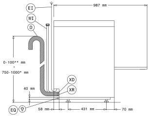
Drain ΕI Electrical inlet (power)
